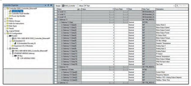
Configuration for Assembly Instances and Size for ODE3 Extended Telegram (4 Words In & 16 Words Out) are as below:
