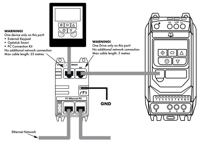
Ground tab – Observe the recommended grounding procedure for the fieldbus network and if necessary, connect this tab to ground where required.
