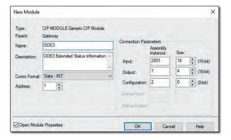
**Step 8.**Device should be added under the CIP Bus
