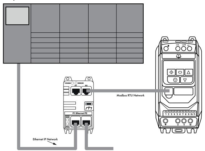
Messages are not sent to the Ethernet Interface, rather they are sent to the drive through the interface. The interface provides a translation from the Ethernet/IP network to the Modbus sub network and therefore to the drive. In order for this to operate successfully, the PLC needs to send the message along with the necessary routing information. This procedure is detailed in the following sections.
