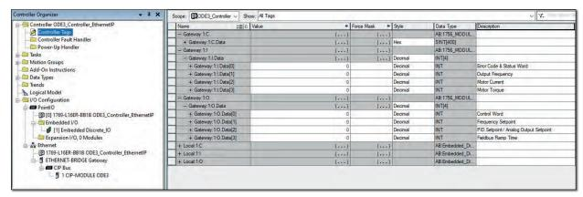
Configuration for Assembly Instances and Size for Standard Telegram (4 Words In & 4 Words Out) are as below:
