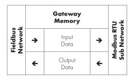
The fieldbus Master can normally be configured to Read and Write the entire gateway memory area in a single transaction, or separate transaction per drive may be configured. The gateway is the pre-configured by Invertek to carry out the necessary individual Modbus RTU transactions to communicate with the Sub Network of connected drives.
