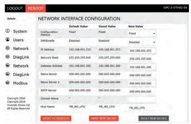
The IP address can be assigned to the module manually by the User (Fixed or Static IP Address) or automatically by the DHCP Server. The default configuration method is Fixed IP address.
