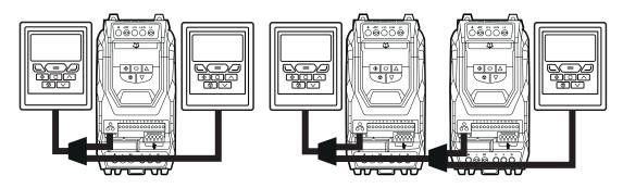
Different drive models can be used on the same Optipad network provided a unique communications address is assigned to each.
